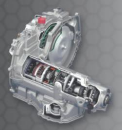
The Ecotec 2.4L I-4 will often be mated with the Hydra-Matic 4T45-E, a dront-wheel drive 4-speed transaxle with a proven record of smooth, smart shifts and rugged durability
