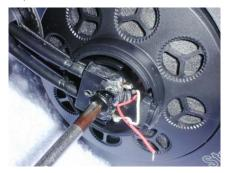
Make sure the wires go through the hole with the protruding rim and put the paper damper back and refit the ring. Mount the assembly back onto the headband and resolder the wires on the right spot. Refit the cap and nameplate.
