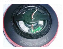
Pull the inner ring upwards and take it off including the paper damper-ring, now you can see the driver and soldering pads.
