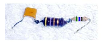
Solder the parallel filter (470  $\mu$ H, 1 $\mu$ F and 39 $\Omega$ ) and the series filter (470  $\mu$ H, 1 $\mu$ F and 56 $\Omega$ ) (see schematic pdf)
