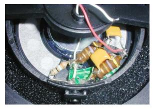
Solder one end of the parallel-filter on the pad where the red wire used to be soldered and the red wire on the other end of the parallel-filter. Then solder the series-filter together with the white wire on the white wire pad and the other end of the series-filter onto the parallel-filter and the red wire.
