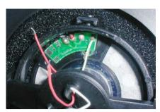
Carefully pry the red wire loose (glued with transparent glue) and desolder it.
